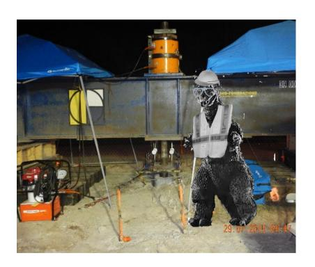
Sacrificial pre-production test piles were loaded to 2000kN
